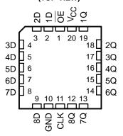
OE does not affect internal operations of the flip-flop. Old data can be retained or new data can be entered while the outputs are in the high-impedance state.
